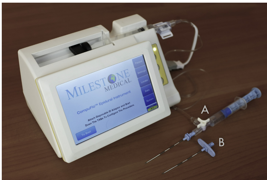
Fig. 1 CompuFlo® set up for (A) Experimental validation (first part of the study) and for (B) Clinical use by trainees (second part of the study). (A) For the validation of the instrument, a three-way stopcock was attached to a standard epidural syringe to let the expert operator perform the epidural block in the usual fashion, independently and unaware of the CompuFlo® flow rate adjustments and pressure recordings. (B) For the second part of the study the CompuFlo® device was attached via the tubing directly to the Tuohy needle, in this case the physician being able to see the CompuFlo® readings and hear the audio
