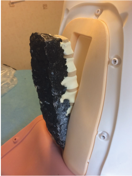
FIGURE 3: The neoprene-silicone mixture used for ligamentum interspinosus and paravertebral muscles (multifidus).
